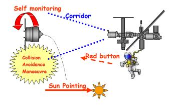
When anything goes wrong, the PFS is in charge of safely moving the ATV apart from the ISS, and to orient it towards the sun ("Collision Avoidance Manoeuvre", CAM)
