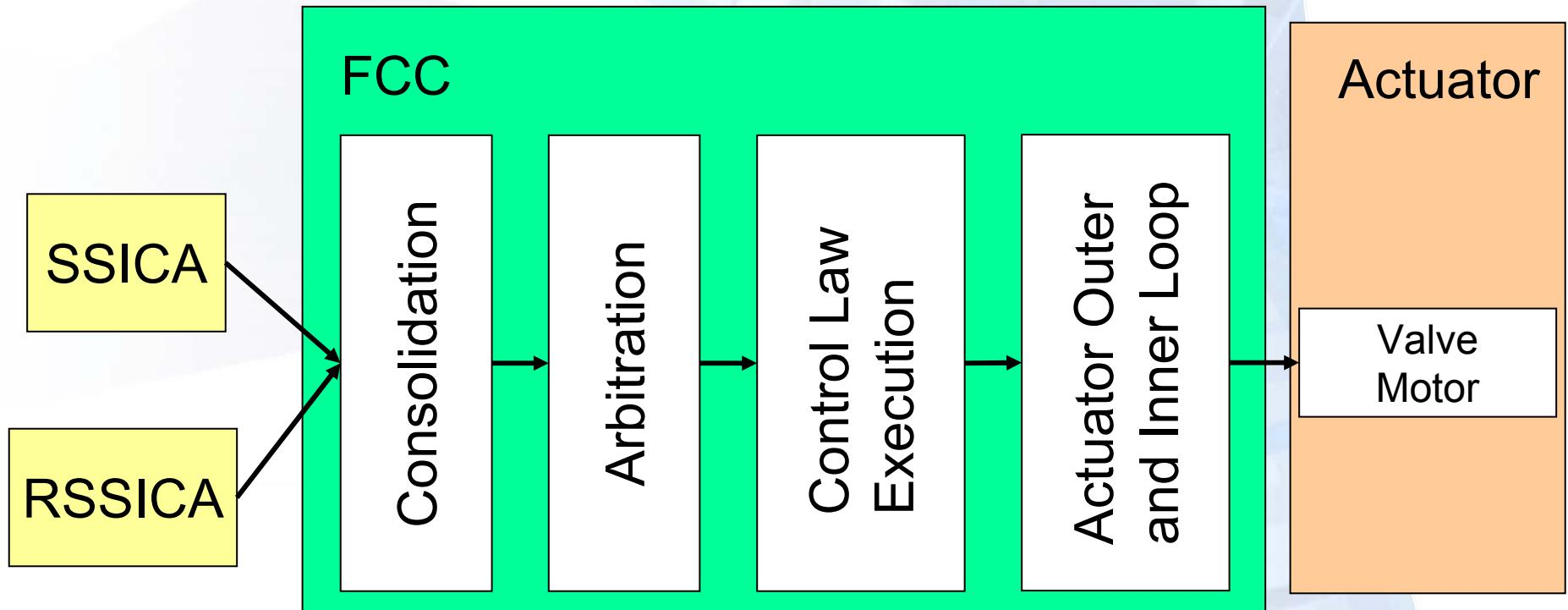
Iteration Rates: 40 Hz; 160 Hz; 320 Hz
