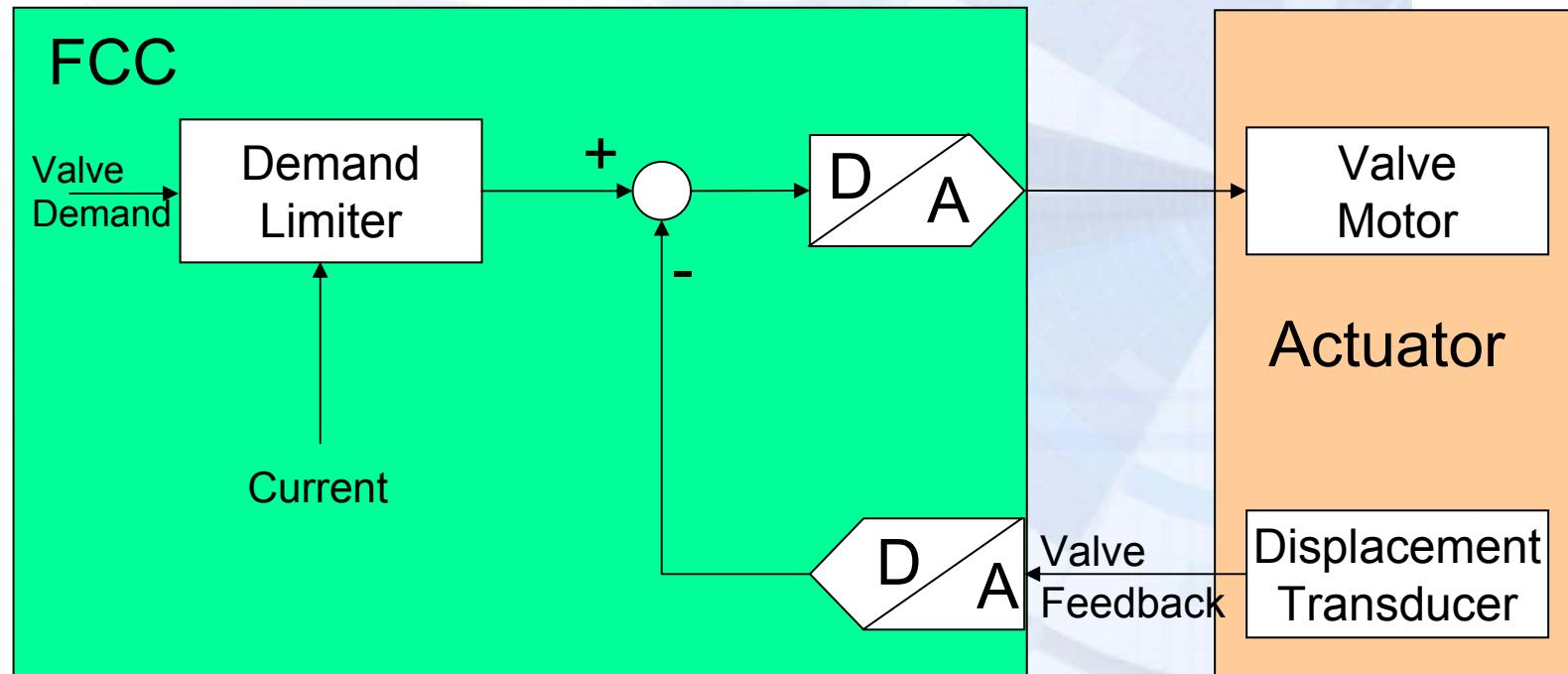
Iteration Rate: 320 Hz
