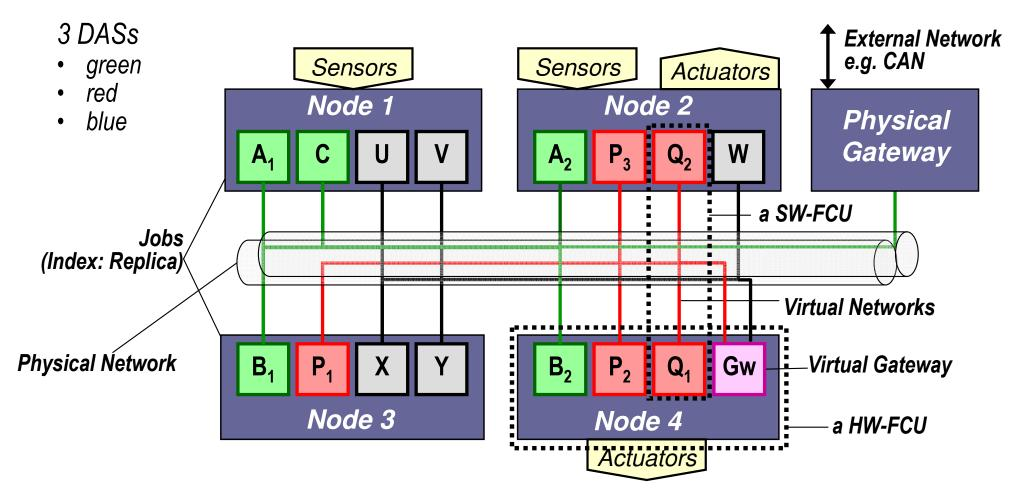
Fault-Containment Units (FCU): Hardware – Node, Software – Job (all replicas)
