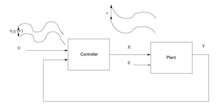
for instance an unstable controller can stabilise an unstable environment.
