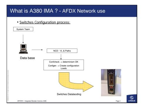
Switch configuration process: the important point is that this configuration is performed at design time; flexibility supports multiple configurations for the aircraft.
