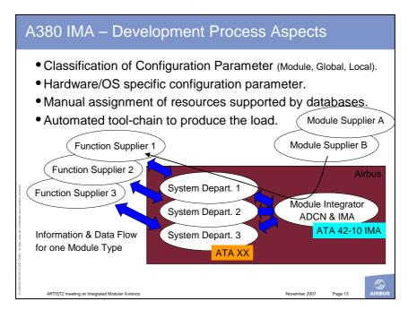
High parallel IMA development process requests formal requirement and design specifications in order to cope with rising complexity of distributed systems. Model based design-space exploration techniques will be needed to analyze and optimize future IMA architectures.
