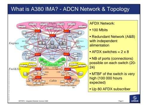
CPIOM + IOM + network + switches, AFDX (Avionics Full Duplex Ethernet), fully compatible with Ethernet; CPIOM allow for uniform handling of all applications; no power supply modules, part of networks or CPIOM  $\rightarrow$  scalability.
