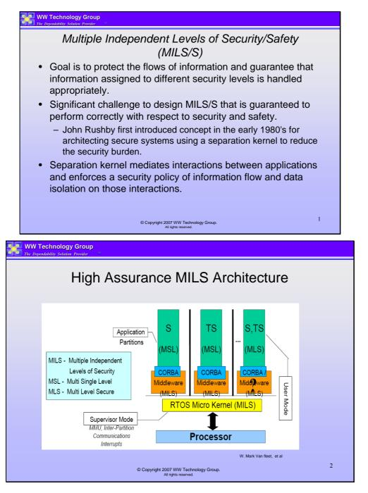
MILS architectures are analyzed using a component-based analysis approach. It is very important to understand the information flows. Certain aspects are analogous to the analysis of error propagation that are available in current version of EDICT but needs some adaptation.
