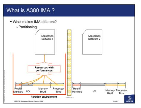
Regarding timing: time slots are allocated to partitions. Memory is protected via MMU to ensure that it remains safe.
