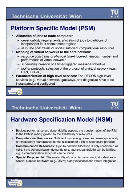
Notes: scheduling is a central activity to ensure and drive the mapping; TDMA multiplexing. This methodology puts emphasis on timing whatever the nature of the application is.
