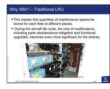
If you look at the communications on past aircraft it is in most cases point to point even where digital data buses were used they were in the main based on ARINC 429 a standard where every sender of information has its own bus and in most cases because of data needs several buses
