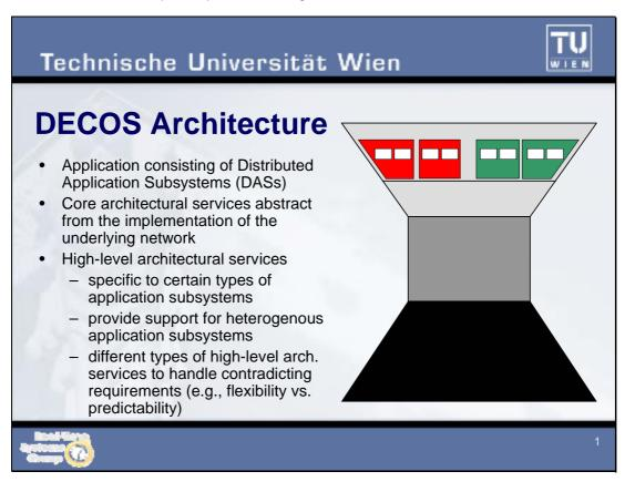
The layered nature allows supporting contradictory features for different uses.
