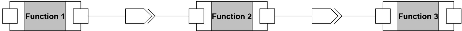
$$t_{RFunction1} + t_{RFunction2} + t_{RFunction3} \neq t_{Rend-to-end}$$
