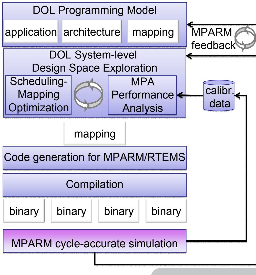
The programming model and high-level API of DOL were ported to the MPARM simulation platform – ***first prototype ready***
