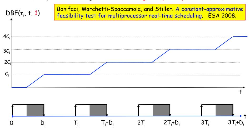
DBF( $\tau_i$ , t, s) = maximum cumulative execution requirement of jobs of sporadic task  $\tau_i$  in any interval of length t, when executing on a speed-s processor (s \le 1)
