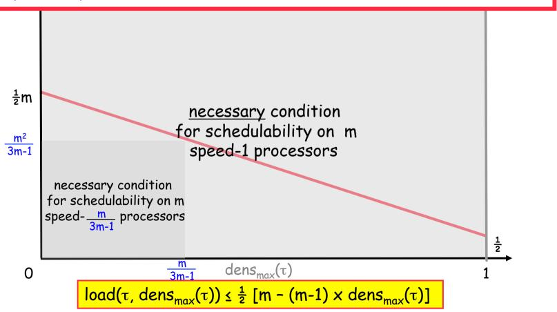
Any sporadic task system schedulable upon m processors is partitioned-EDF schedulable on m processors that are each (3-1/m) times as fast
