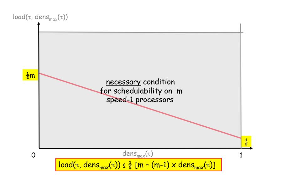
Any sporadic task system schedulable upon m processors is partitioned-EDF schedulable on m processors that are each (3-1/m) times as fast
