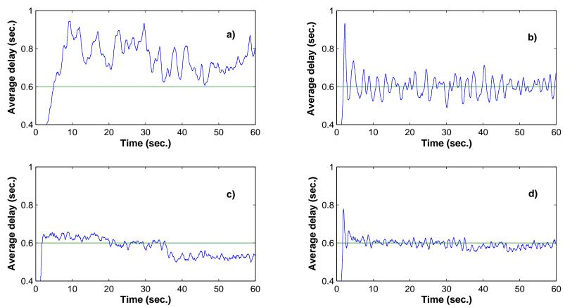
• a: M/M/1, b: M/M/1 + PI, c: Predictor d: Predictor + PI
