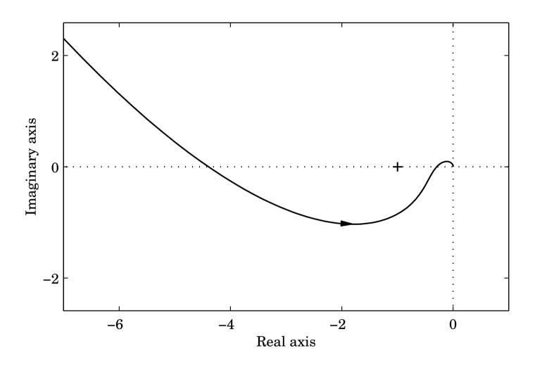
First crossing at  $\omega_1 = 0.162$  rad/s. Predicts limit cycle with period 39 s and amplitude  $A_1 = \delta/2$ .
