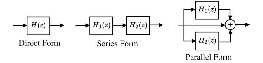
Try to balance the gain such that each subsystem has about the same amplification
