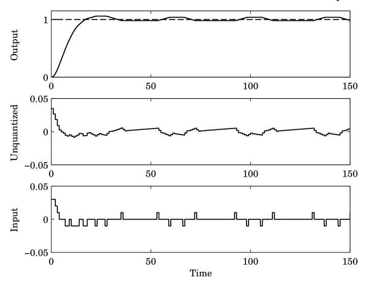
Limit cycle in controller output with period 39 s, amplitude 0.005
