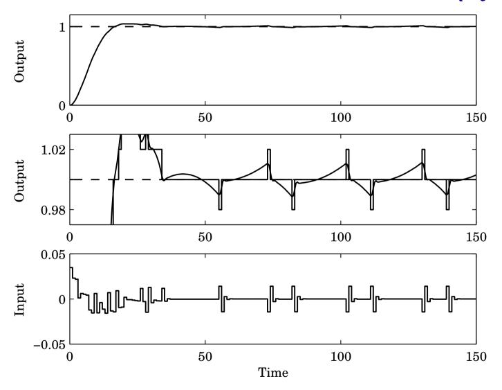
Limit cycle in process output with period 28 s, amplitude 0.01
