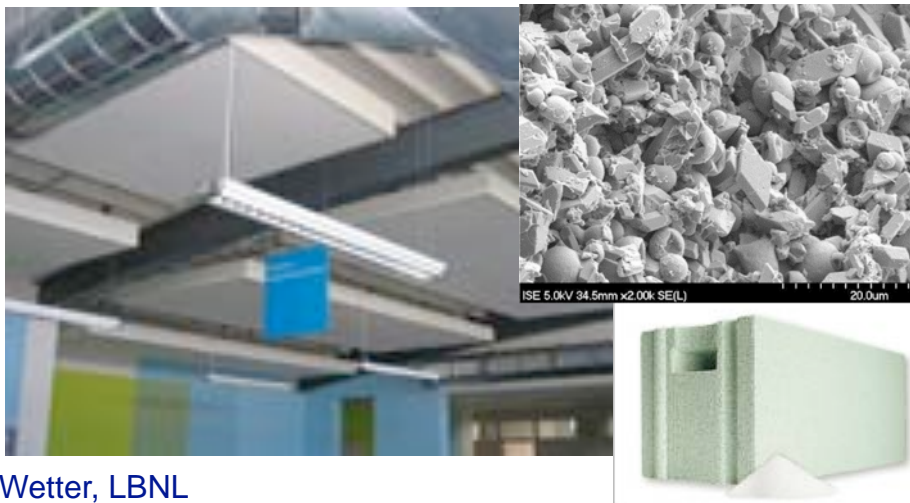
Phase change material to increase thermal storage
