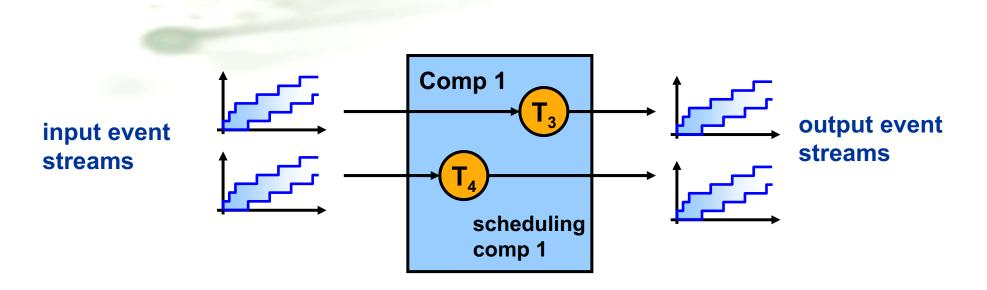
Output event model of one processor becomes input event model of successor → compose multiple local analyses into system level analysis
