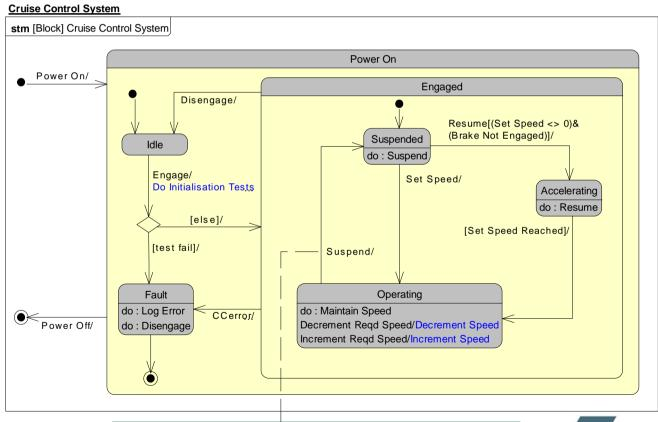
Suspend operation also called when brake applied or when throttle applied for >20 sec
