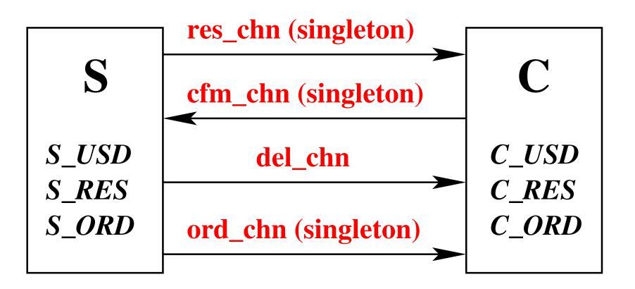
inv2\_1: $C\_USD \subseteq PRD$ inv2\_2: $C\_RES \subseteq C\_USD$ inv2\_3: $C\_ORD \subseteq C\_RES$
