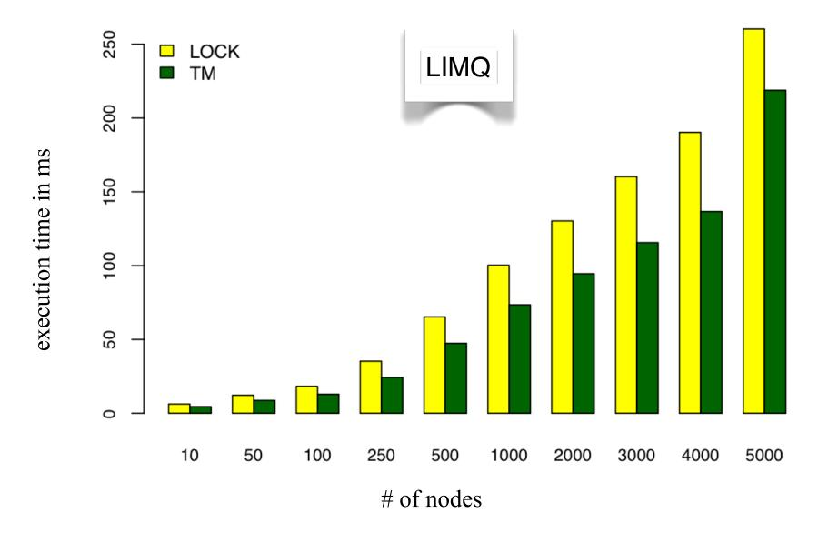
Running on JOP with 4 cores, each JOP core has a local 4 KB instruction cache and 1 KB stack cache. Using Altera DE2-70 Development board with Cyclone II EP2C70 FPGA.
