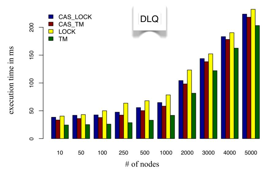
Running on JOP with 4 cores, each JOP core has a local 4 KB instruction cache and 1 KB stack cache. Using Altera DE2-70 Development board with Cyclone II EP2C70 FPGA.
