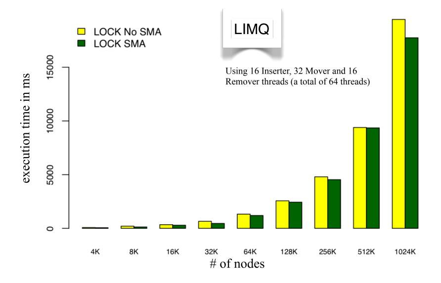
Running on an Azul Vega 3 3310B, with two 54-core processors and 48GB of RAM, on top of the Azul Virtual Machine with the Concurrent Pauseless GC.
