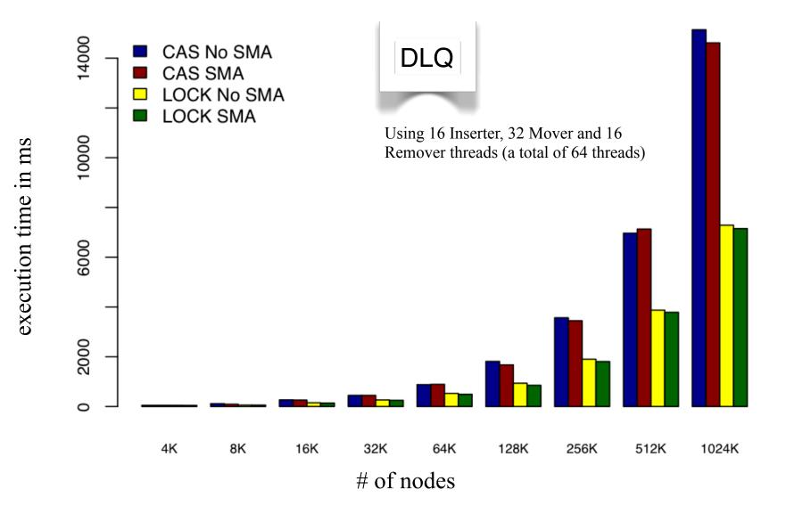
Running on an Azul Vega 3 3310B, with two 54-core processors and 48GB of RAM, on top of the Azul Virtual Machine with the Concurrent Pauseless GC.
