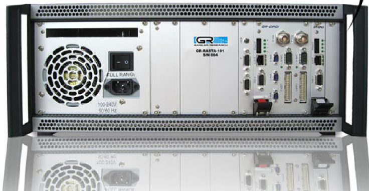
GR-RASTA - LEON2/3/4 spacecraft avionics development platform. Source: Aeroflex Gaisler .
