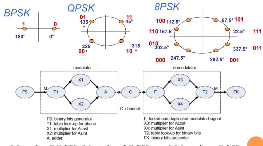
• M=1 for BPSK, M=2 for QPSK, and M=3 for 8PSK
